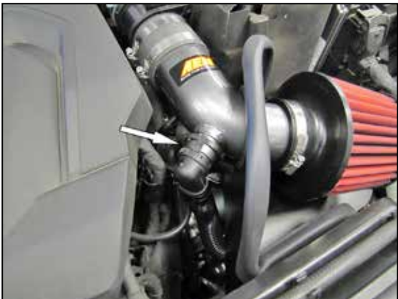
19. Connect the air injection hose to the AEM® intake tube.
