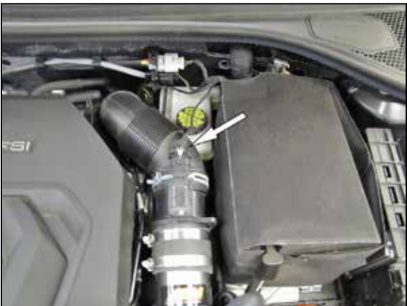
20.Reconnect the mass air sensor electrical connection.
